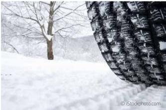
As important as having good tyres is taking good care of them. This covers such aspects as ensuring that they are inflated to the correct pressure, are not worn out, have the minimum tread depth, and are appropriate for the climatic conditions in which they are used.
