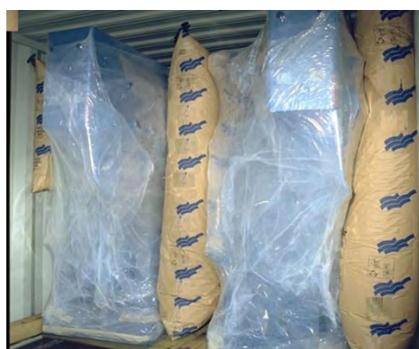
Figure 7.10 Irregular shaped packages blocked with dunnage bags
