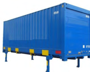
Figure 5.6 Swap body landed on support legs
