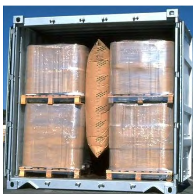
Figure 7.9 Gap filled with a central dunnage bag
