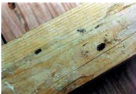
Figure 6.13 Wood frass from boring insect
