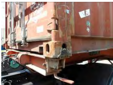
Figure 6.2 Mud in corner fitting
