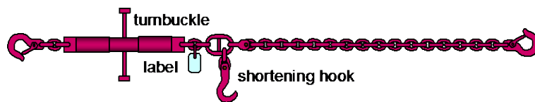
Figure 7.18 Standard chain lashing with shortening hook
