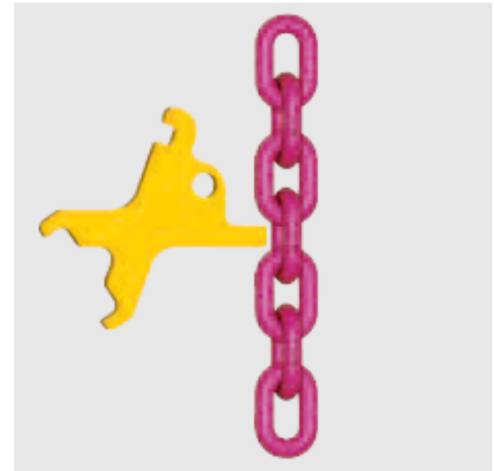
Testing elongation of pitch caused by wear of nominal diameter
