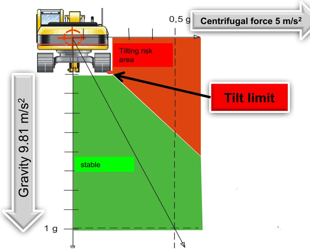
In order to determine tilting risk, we plot the acceleration forces (Gravity = 1 g = 10 m/s<sup>2</sup> (9.81 m/s<sup>2</sup>) = 10 cm) / lateral; maximum acceleration 0.5 g = 5 m/s<sup>2</sup> = 5 cm) using lines. Then, both lines are extended down and to the right until they meet (parallelogram of forces).
