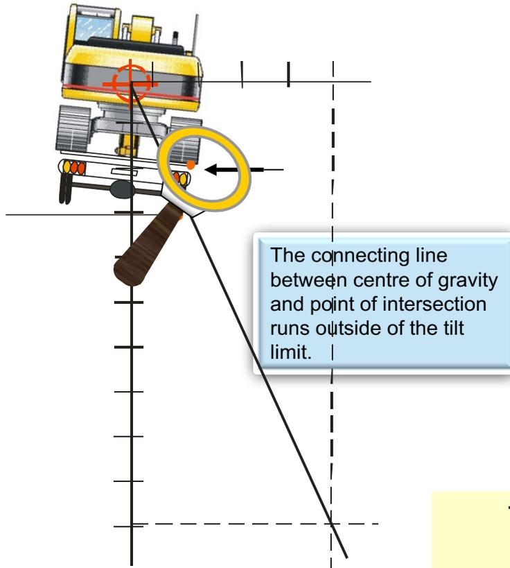
Through the loading of the crawler excavator, there is a shift of the tilt limit to the inside, towards the centre of gravity.
