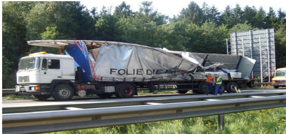
Cargo can shift and deform the vehicle body
