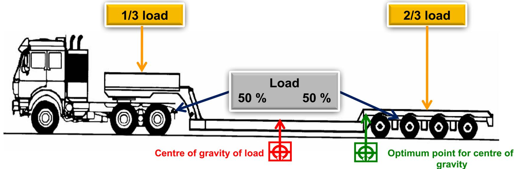
Particularly when using combinations with drop-deck trailers without interposed chassis, there is often a considerable exceedance of rear axle load of the transfer truck, even if the maximum total weight of the rig has not yet been exceeded.
