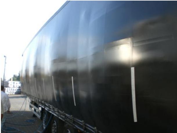
Side wall test with 10,595 daN, maximum elastic deformation 300 mm
