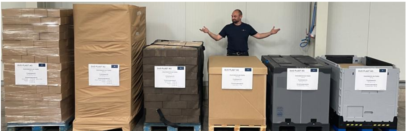
Figure 2-1: Picture of different transport packaging systems (from the left to the right: single-use stretch wrap, single-use paper stretch, reuse sleeve, single-use and reuse cardboard box, reuse plastic box type A and type B)
