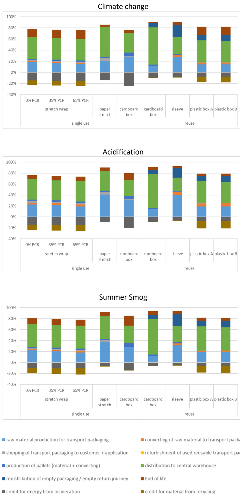
Figure 4-12: relative contribution of lifecycle steps for the impact categories Climate change, Acidification and Summer smog in the application field buckets
